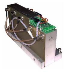
Olson Technology, Inc.'s SpectrumPlus Return Path Bandwidth Expansion System is a reliable, field-proven and cost-effective family of products which consolidates and transports up to 32 separate, phase-locked 5-42 MHz upstream signals per singlemode fiber to the receive system site, vastly enhancing network capacity and ultimately decreasing network complexity.
