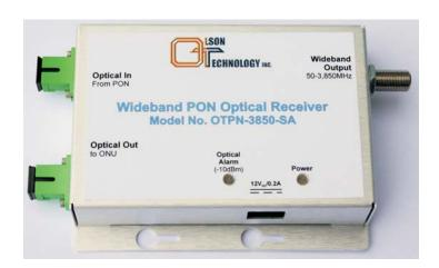
The Olson Technology, Inc. **Model OTPN-3850-SA** provides 50-3,850 MHz bandwidth, allowing it to carry CATV signals from 50-870 MHz along with two stacked 950-2,150MHz L-Band signals. The L-Band signals are usually at a level below the CATV signals.
