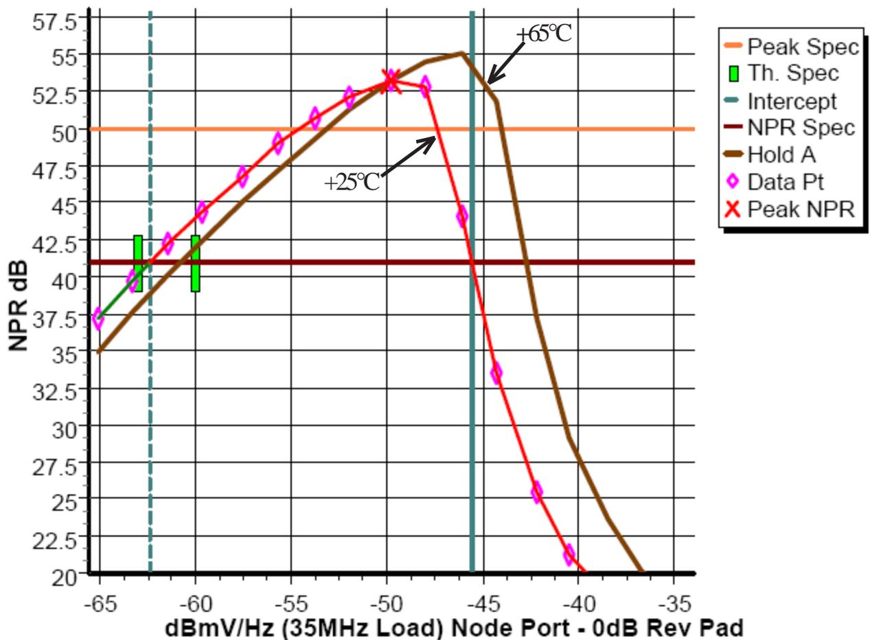
Figure 5 - SA6940 Typical NPR Curve
