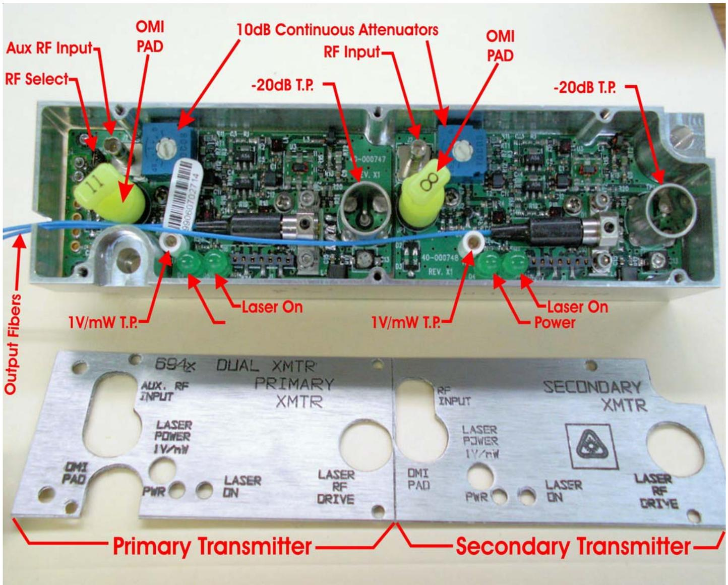
Figure 3 - Inputs, Outputs, Controls & Indicators on the SA6940-RT
