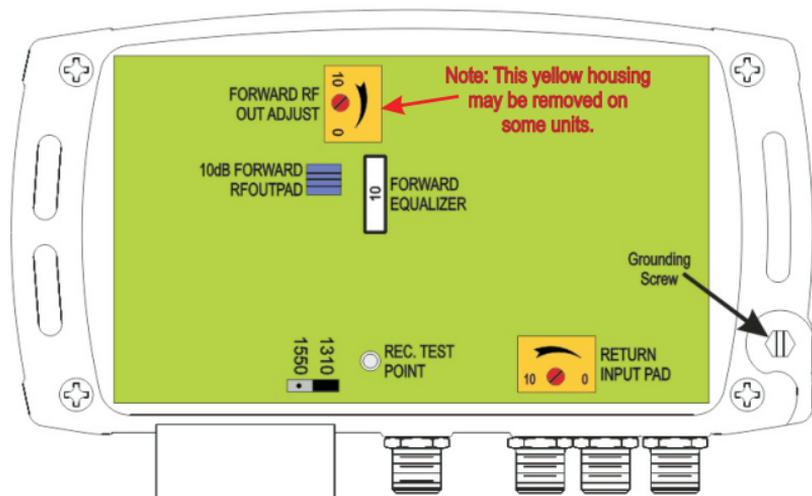
**Figure 3 - OTPN-800CH Location of Internal Adjustments**
