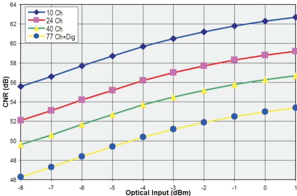
Figure 2 - Typical CNR vs. Optical Input Level
