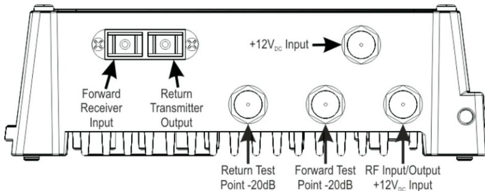
**Figure 1 - OTPN-800CH Inputs and Outputs**
