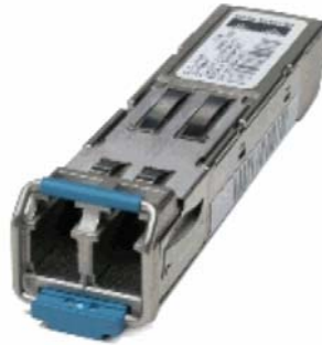
Typical Mating SFP Module
