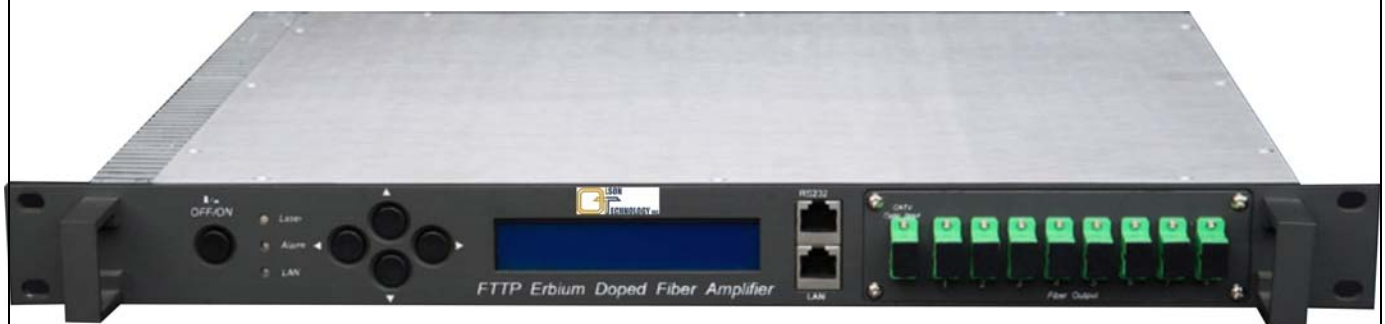
1RU Model - Combined Output Power up to 1,000mW (+30dBm)
