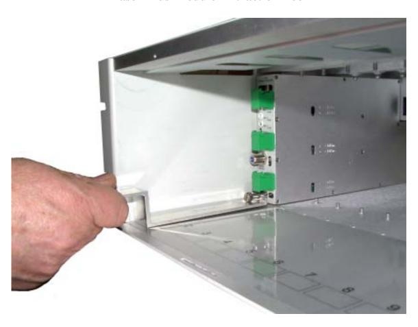
Insert module puller and slide the notched end underneath the pull tab on the front of the inserted module as shown above. Then press down on the handle, this will lift the notched end thereby lifting the front of the module. Then proceed by pulling the unit out while pressing down on the handle.
